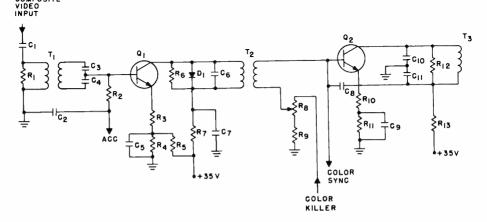
Fig. 9. A two-stage transistor color i-f amplifier.
