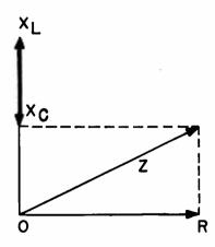
Fig. 5. Vector addition of a 10-ohm resistance, a 10-ohm inductive reactance, and a 5-ohm capacitive reactance.
