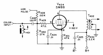
Fig. 8. Schematic diagram of a burst-gate amplifier stage.
