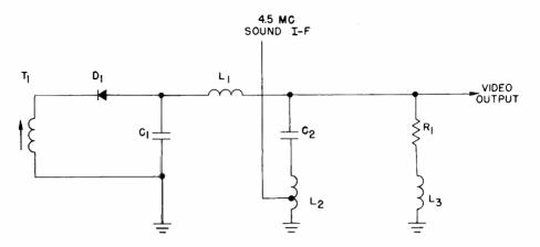
Fig. 2. A typical video detector from a monochrome receiver.
