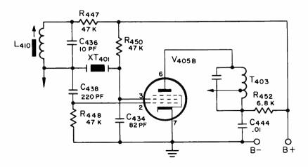
Fig. 7. Schematic diagram of a color oscillator.
