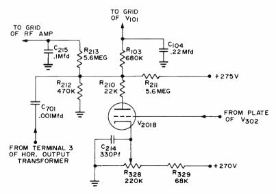
Fig. 6. Diagram of a keyed agc amplifier stage.
