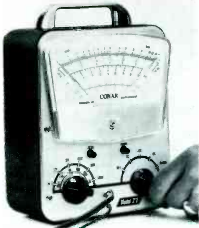
Fig. 1. The CONAR Model 211 VTVM, built in the second demonstration kit.
