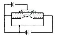
Fig. 6. Current flow through an Nchannel IGFET with bias applied.
