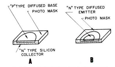
Fig. 1. Forming base (A) and emitter (B) in the planar process.
