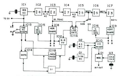
Fig. 6. Block diagram of the CONAR Model 680 Color Generator.
