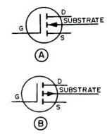
Fig. 8. The schematic symbols for the enhancement type of IGFET's. (A) An N-channel unit; (B) a P-channel unit.
