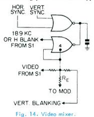
to the IC mixer to eliminate video pulses
