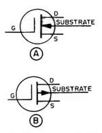
Fig. 7. Insulated-gate field-effect transistors. (A) The schematic symbol for an N-channel unit; (B) the symbol for a P-channel unit.
