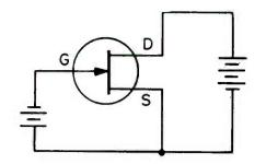
Fig. 2. Schematic representation of the circuit shown in Fig. 1.
