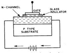
Fig. 5. Current flow through an insulated-gate, N-channel field-effect transistor with no bias applied.
