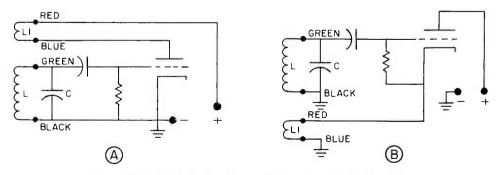
Figure 4. Plate feedback is shown at A; cathode feedback, at B.
