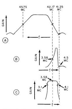
FIG. 2. The color i-f response (B) is shaped to compensate for the unequal response above and below 42.17mc in the video i-f response (A) to produce a flat-topped overall color sideband signal response (C).
