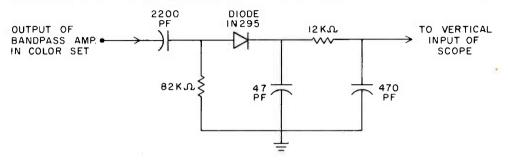
Figure 5. Detector circuit for demodulating the swept signal.
