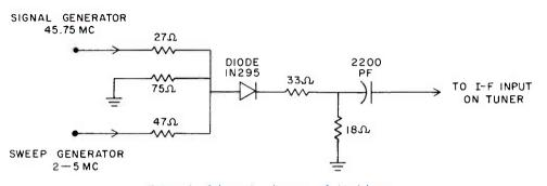
Figure 4. Schematic diagram of Modulator.
