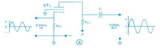
Figure 10A. With the grounded grid circuit there is gain but no phase reversal.
