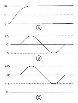
Fig. A illustrates a typical dc voltage. Notice that it begins at zero and rises to a maximum constant value. Fig. B shows a typical ac voltage. It begins at zero and rises to a maximum positive value, returns to zero, reaches a maximum negative value, and returns to zero again.
