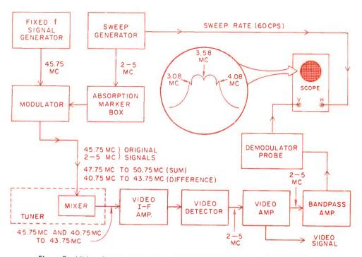
Figure 3. Video Sweep Modulation alignment system shown in block form.
