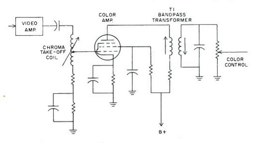
Figure 7. Bandpass amplifier circuits of a typical color receiver.
