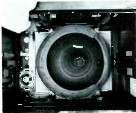
Fig. 3. In this receiver, the picture tube is held in the cabinet by the shield which is secured by four nuts.
