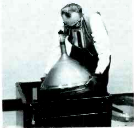
Fig. 4. The picture tube must be tilted slightly so it will clear the cabinet edges of this receiver.
