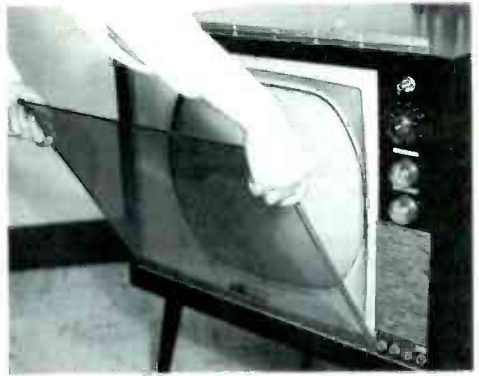
Fig. 8. The lower edge of the safety glass fits into a channel in the cabinet.
