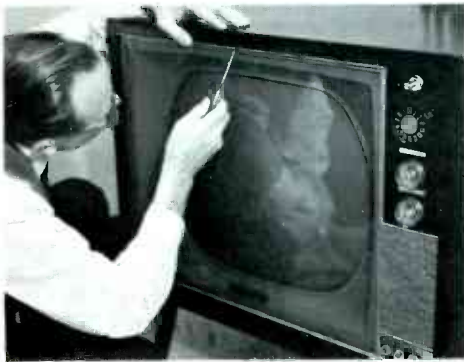
Fig. 7. A removable trim strip secures the safety glass to the cabinet.
