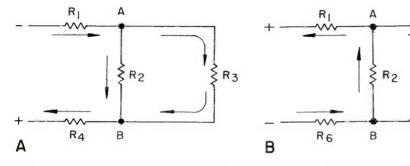
Fig. 3. Identifying various circuits by assigning polarity designations and tracing the path of current flow.
