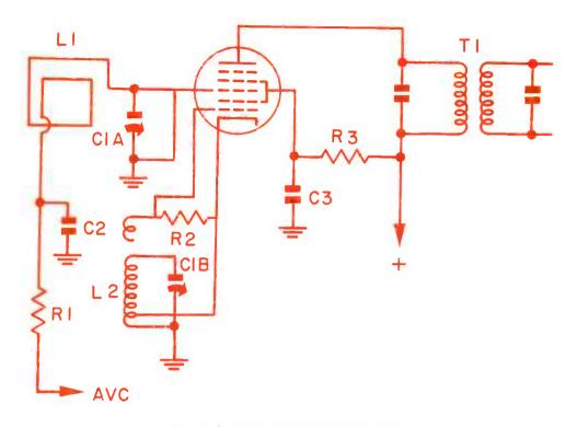
Fig. 4. A typical mixer-oscillator stage.
