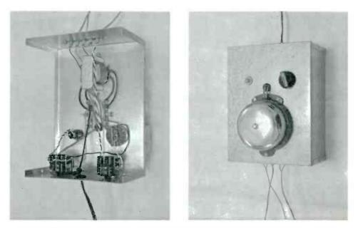
Fig. 10. (A) Inside view of 3-way shop protector; (B) Outside view of 3-way shop protector.
