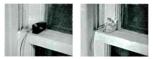
Fig. 9. (A) Microswitch installed on window; (B) Foil strip window switch.
