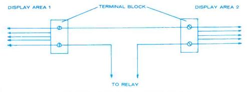
Fig. 4. Connecting two or more terminal blocks.
