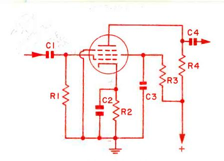
Fig. 1. A typical pentode stage.
