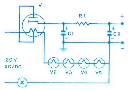
Fig. 5. A typical ac-dc power supply.
