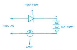
Fig. 11, Simple battery charger.
