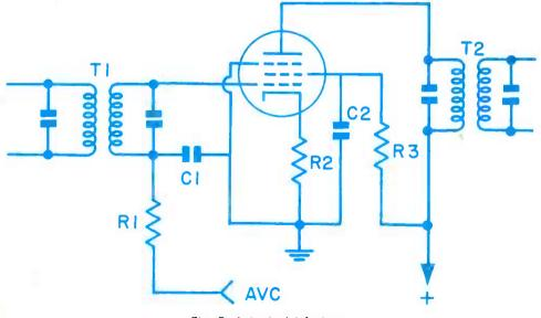
Fig. 3. A typical i-f stage.
