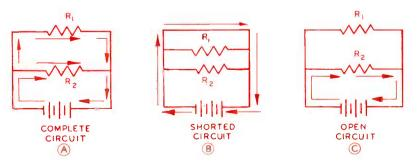
Fig. 1. Differences between an open circuit and a short circuit.
