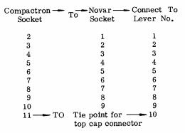
When using a tube chart in setting up your tester to check compactrons, use this table to locate the proper levers for various electrodes. Also remember there are no levers to throw for filament power.
