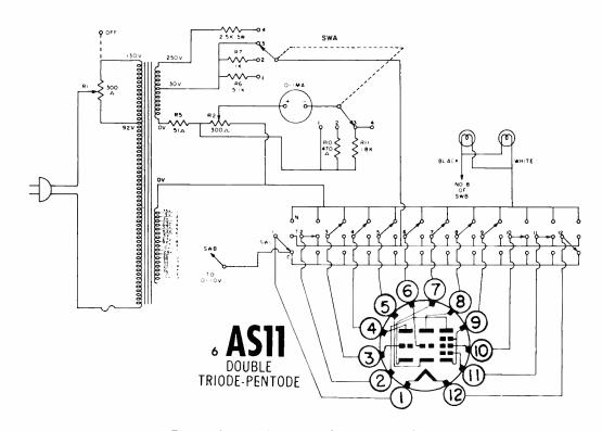
Fig. 6. Testing the pentode section of a compactron for emission.
