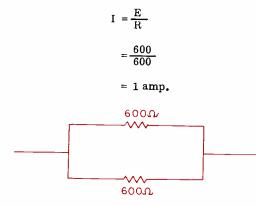
Fig. 8. Find value of two resistors in parallel.
