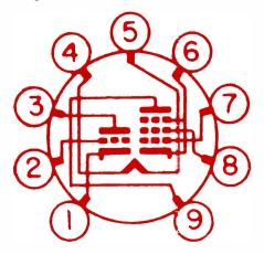
Fig. 1. Base layout of a triode-pentode type tube.
