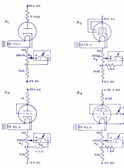
Fig. 7. Basic setups to check cathode emission.
