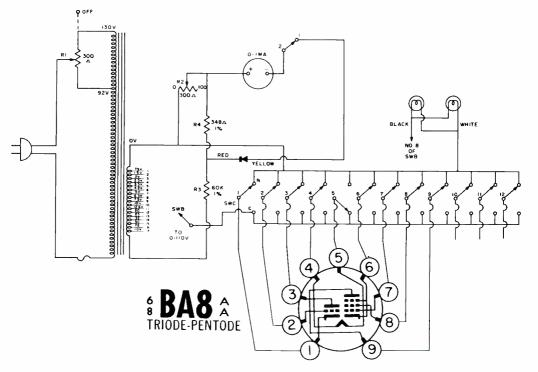
Fig. 4. Setup for line voltage adjustments and filament voltage.
