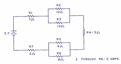
Fig. 10. Find the applied voltage E in the circuit shown.
