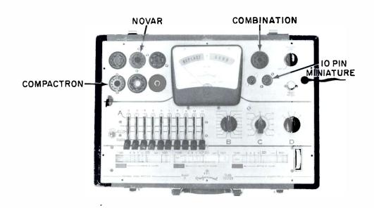
Photo of a modernized old tube tester.
