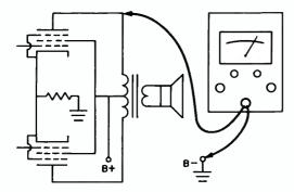
FIG. 5. The VTVM as an AC voltmeter may be connected from either plate to chassis. The sound from the loudspeaker can be kept fairly low with the attenuators.
