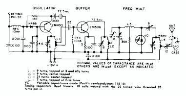
The OSCAR transmitter circuit.
