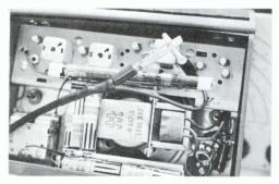
FIG. 10. Closeup showing how hot and ground leads of the 280 are clipped together and slipped over a loopstick in a transistor set.
