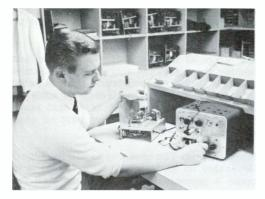
FIG. 8. Technician Jim Johnson of NRI's Quality Control calibrates an assembled 280 Signal Generator by beating its signals against a special crystal-controlled standard.
