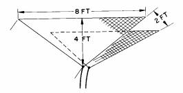
FIG. 3. Design for a "short-horn" antenna.
