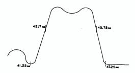
FIG. 3. Response curve of a typical video i-f in a color receiver.
