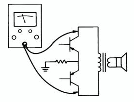
FIG. 6. The VTVM set for AC measurements may be connected to the collector leads of output transistors, or you can get by with a smaller signal from either collector lead to chassis.
