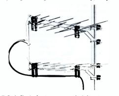
FIG. 6. Stacked antennas provide 3 db extra gain.
