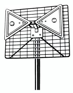
FIG. 3. Bowtie-with-screen type outdoor UHF antenna.
