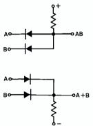
and operate like this. In the case of the AND gate, if an input appears at A and B, an output will be present. If A appears but B does not, no output. The OR gate gives an output for either A or B.
