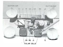
FIG. 4. Wiring of receiver with solar cells shown in lower center. The four suction cups to hold the radio against the window pane are seen at the corners. the signal to the base of Q2. Tie the collector terminal to the other side of J1.
