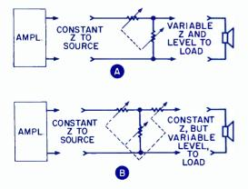
FIG. 4. Variable audio pads: (A) L-pad; (B) T-pad.
