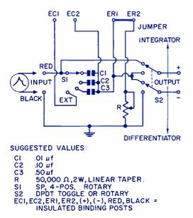
FIG. 1. Circuit of the diffegrator.
