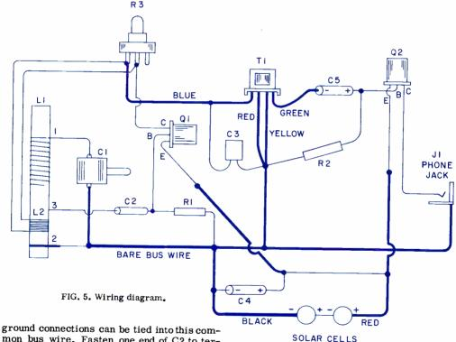
mon bus wire. Fasten one end of C2 to terminal 3 of L1 and the other end to the base connection of Q1. You can identify the transistor connections from Fig. 6. A 1.2-megohm resistor (R1) ties also from this point to ground. Run the two enameled wires from the coil you wound on the loopstick to R3. Be sure to scrape the enamel from the wire and tin the ends with a soldering iron. Wire in the primary and secondary of T1 to their components. Blocking capacitor C5 couples
