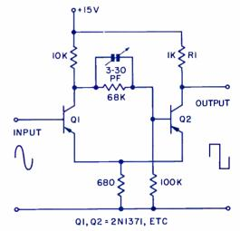
FIG. 6. Transistorized clipper producing square waves from sine wave input.
