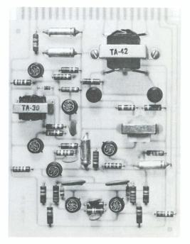
FIG. 5. Printed circuit board of Howler.
