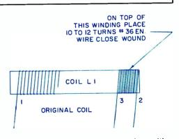
FIG. 3. Extra turns are placed in the position shown for feedback.
