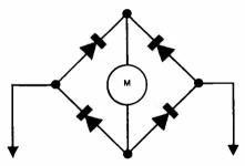
One very important thing to remember when using a rectifier type AC meter, is that the instrument was calibrated on a sine wave and any harmonic distortion will cause inaccurate readings. Another point in passing - always give a quick calibration check when turning on your meter before measuring AC. Measure the power line voltage. This varies a few volts, but will tell you in an instant that all of your rectifiers within the meter are still good.
