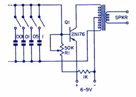
FIG. 5. A simple audio oscillator.
