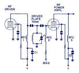
FIG. 5. Use of rf chokes in transmitter.
