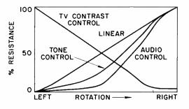
FIG. 2. Potentiometer tapers.
