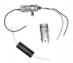
FIG. 4. Power-supply filter capacitors.
