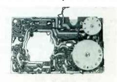
FIG. 2. Bottom view of chassis shown in Fig. 1, showing printed circuit board and circuitry.
