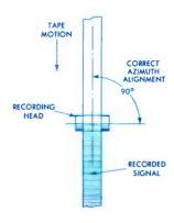
Recording and playback heads must be exactly perpendicular to motion of tape (as shown in the right hand sketch), for minimum distortion and maximum frequency response.
