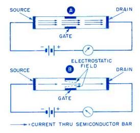
FIG. 2. The current flow through the bar from source to drain is due to the field effect.
