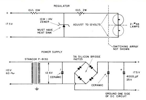
FIG. 3. Surge reducer for complicated lamp arrays.
