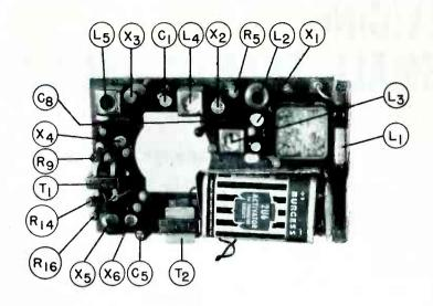
FIG. 1. Top view of the chassis of a transistor portable receiver sh
