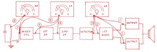
FIG. 5. How to use a signal generator to find a weak stage in a transistor set. The output of the signal generator is set to the correct frequency and moved from stage to stage to check loss in gain.
