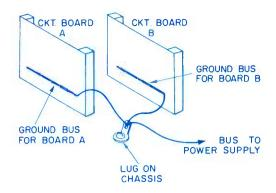
FIG. 5. I wo circuit boards showing common bus for each board. Note that boards and power source are referenced to a central point to eliminate circulating chassis currents.
