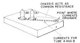
FIG. 1. An illustration of a chassis showing current flow through common area of metal.
