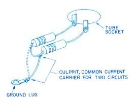
FIG. 4. Resistors connected between tube circuits and ground lug showing source of ground problem. The dotted line indicates a possible method of correcting the problem.
