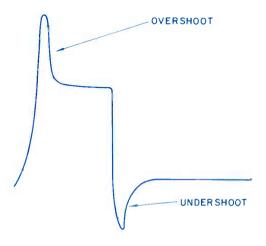
FIG. 3. Pulse with overshoot and undershoot caused by circulating ground currents. Pulse should have characteristics shown in FIG. 2B.
