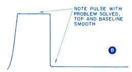
FIG. 2. (A) Pulse with damped oscillations on top and baseline. (B) Corrected pulse.
