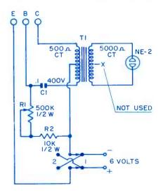
FIG. 3. The switch is thrown to the right for PNP transistors and to the left for NPN's.
