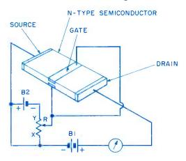
FIG. 1. The construction of a FET is different from that of an ordinary transistor.
