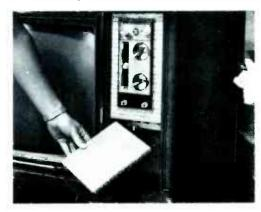
The bottom half of the right hand panel is removable to reveal the color convergence controls.
