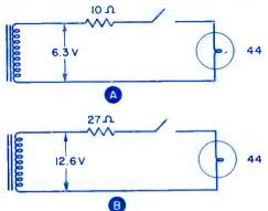
FIG. 1. Circuits for reducing turn-on surges by use of series resistor.
