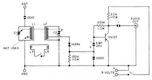
FIG. 5. The circuit of an AM tuner capable of providing top quality reception. C1 and C2 are 365 mmf variable (ganged). L1 and L2 are loopsticks (Allied Radio No. 91-C-057 or equiv.).
