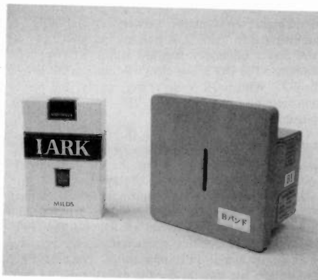
FIGURE 8: External appearance of practical FPU transmitter.
