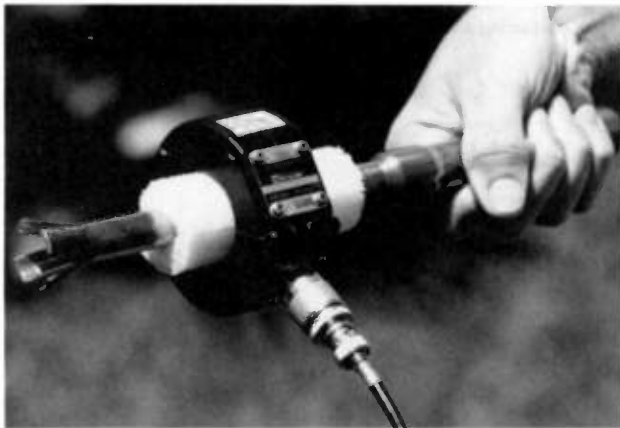
Figure 4. Photograph of the current probe assembly used to measure contact currents.
