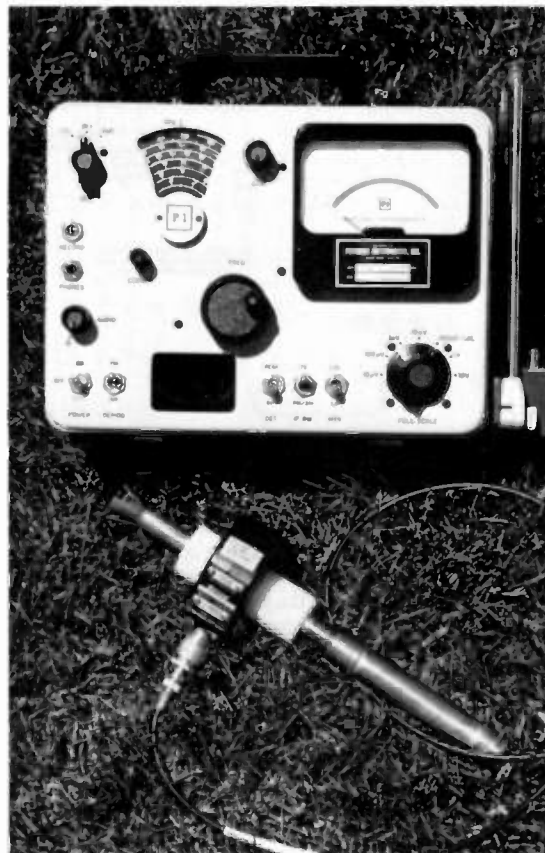
Figure 5. Photograph of the current probe assembly and field strength receiver used to measure contact currents. The receiver is used as a sensitive tuned voltmeter for detecting the RF output voltage from the current transformer.
