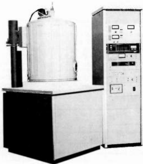
FIGURE 3. COLLECTOR ELECTRODE COATING EQUIPMENT
