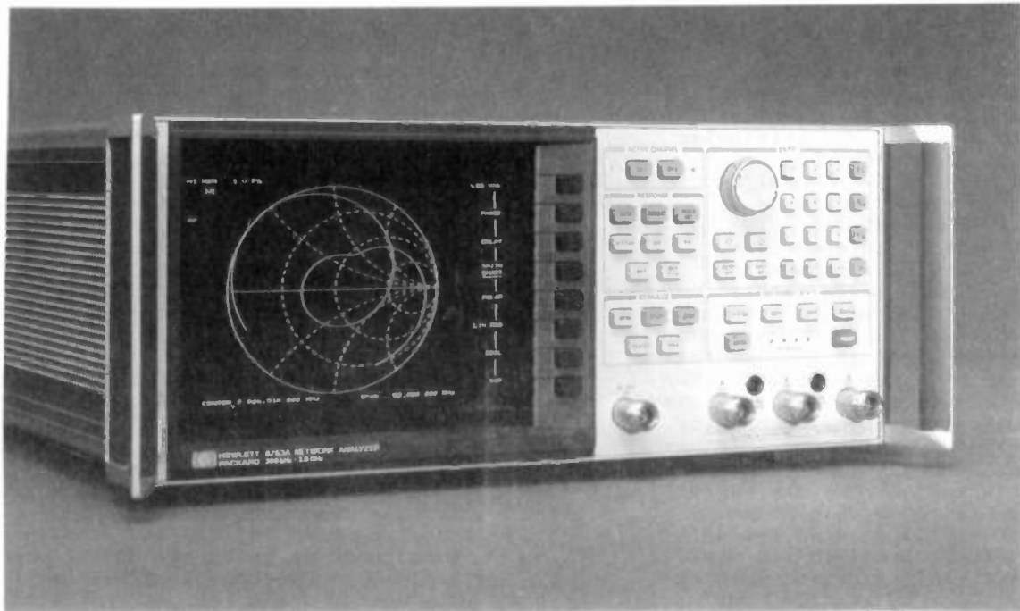
Figure 1 Hewlett-Packard Model 8753A Network Analyzer
