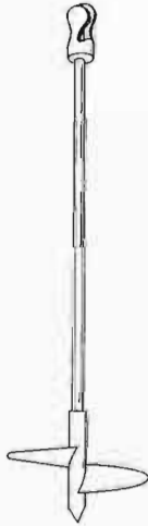
Fig. 59. Screw-type earth anchor.
