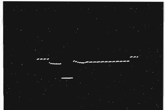
Fig. 74. Positive streaking—window signal—expanded vertical.
