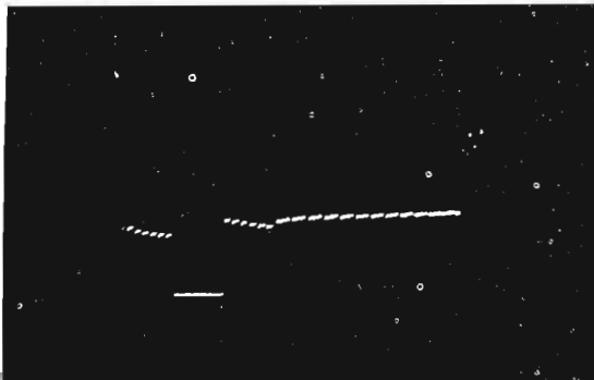
Fig. 86. Smearing—test pattern—expanded vertical.
