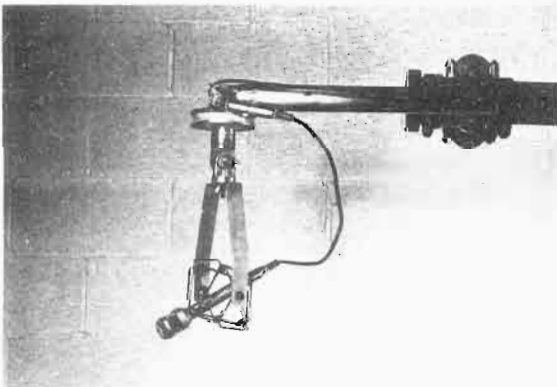
Fig. 39. Shows a boom microphone with the normal rubber band type mount.
