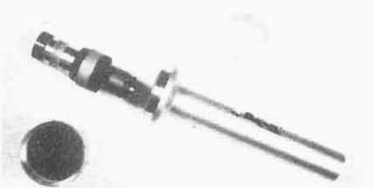
Fig. 37. New microphones showing the internal construction where a rubber isolation doughnut is used.
