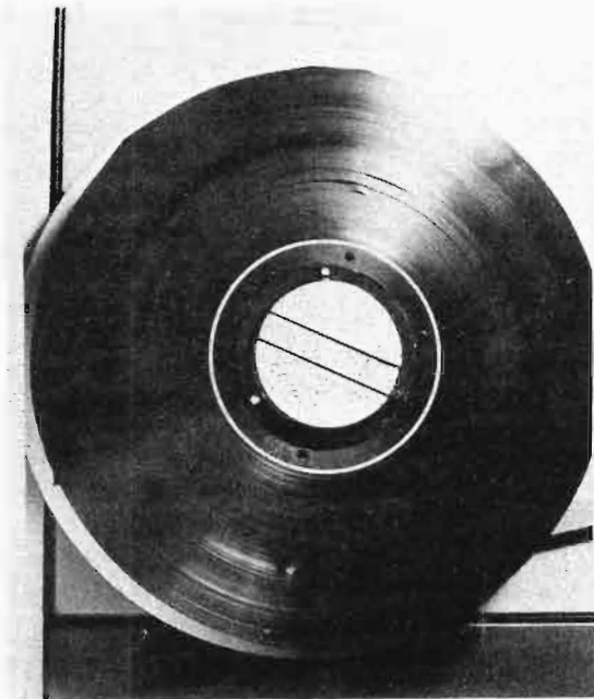
Fig. 50. Video tape "cinching."
