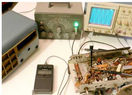
The first IF primary winding of a Hallicrafters 5R34A "Continental" resonates at nearly 800 kHz indicating a seriously degraded silver mica capacitor but good coil.
