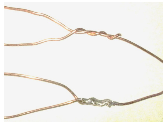
View of two loop "knots," before and after soldering. Get the joint good and hot and flow plenty of solder into nooks and crannies. (Photo by author)
