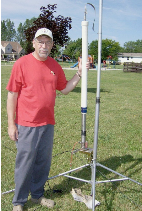
Larry Parker VA3EDY shows off one of his home-brew, multi-band mobile/portable HF antennas for Field Day. Note the high-tech antenna mount made from a discarded aluminum clothesline!
