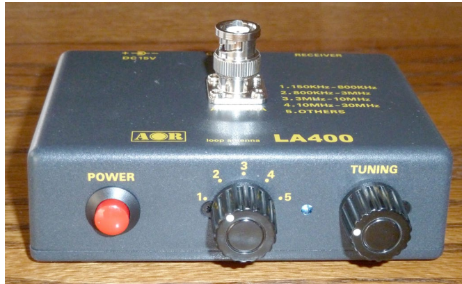
AOR LA400 Active Antenna Control Box – The control box has a front panel power switch, band switch, and fine tuning control. A BNC connector atop the case permits direct loop attachment or accommodation for a remote cable
