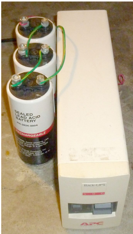
Photo C UPS With High Capacity External Battery
