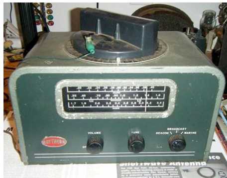
Reader Mike Martel is seeking any user documentation for this Raytheon GM 114B RDF receiver (photo courtesy Mike Martel).
