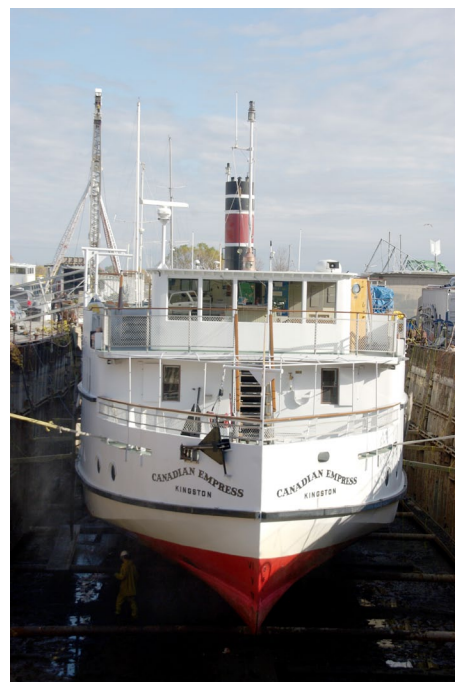
MV Canadian Express in dry-dock for inspection before winter layup and maintenance.
