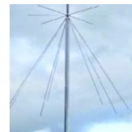
One of the popular broadband discone antennas, touted to cover 25-1300MHz. Ten and six, anyone? (Photo courtesy mjjenterprises.com)
