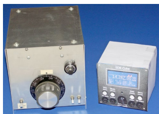
On the left is a Kenwood TS-120S VFO I packaged (somewhat crudely) in 1993. On the right is a life-size mock up of a Midnight Design Solutions SDR Cube monoband transceiver, complete with DDS, software-defined innards, built-in DSP controller, band scope and digital display! (NT0Z photo)
