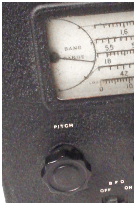
Before the dial plate could be taken off, both indicating needles would have to be removed.
