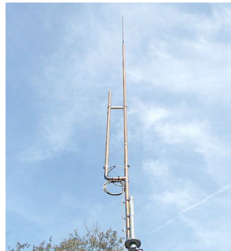
KK4BCV's elegant J-pole vertical for 6 meters is just 16 feet tall. (Photo courtesy hamuniverse.com)
