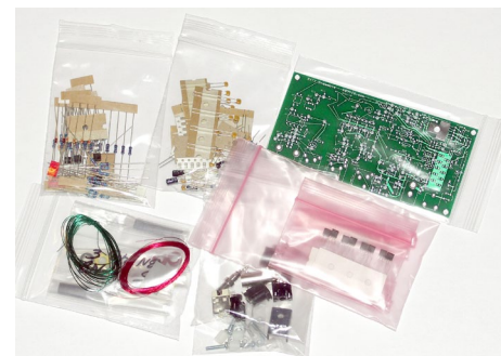
One of the kits I’m working up the nerve to build this fall is a three-band Sofrock RXTX Ensemble SDR transceiver. (NT0Z photo)
