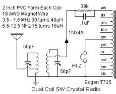
The MT Special Dual Coil Shortwave Crystal Set Schematic.
