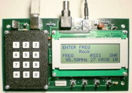
The Shortwave Daddy is built around a professionally-laid-out PC board utilizing high quality components. All factory pre-drilled holes are "through hole" making soldering a more reliable process. The few connections for surface-mount connections, and the surface-mount parts themselves, are solder-plated for more secure attachment.
