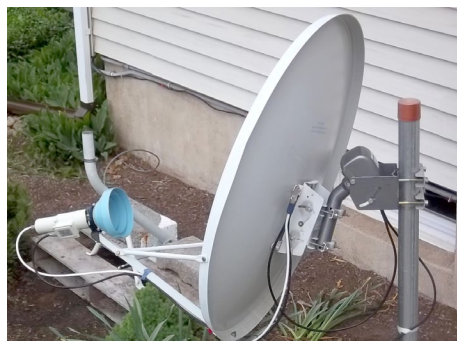
BSC621-2D C/Ku band universal LNBF with offset bracket and 100 cm dish. (Courtesy: Mario Filippi N2HUN)
