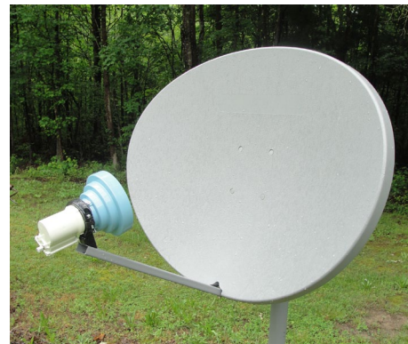
Channel Master 84E 40 inch offset fed Ku-band dish set up for C-band reception. (Courtesy: Author)
