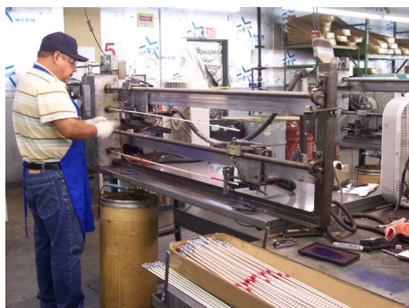
Photo A - Winders for the fiberglass whips
