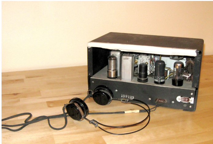
Hallicrafters S-38B radio showing tubes and original Trimm headset.
