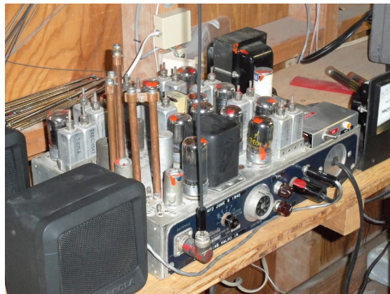
Motorola DeLux 30D receiver from 1947 (Courtesy: Author)
