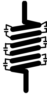
Figure 1 - Distributed capacitance in a coil
