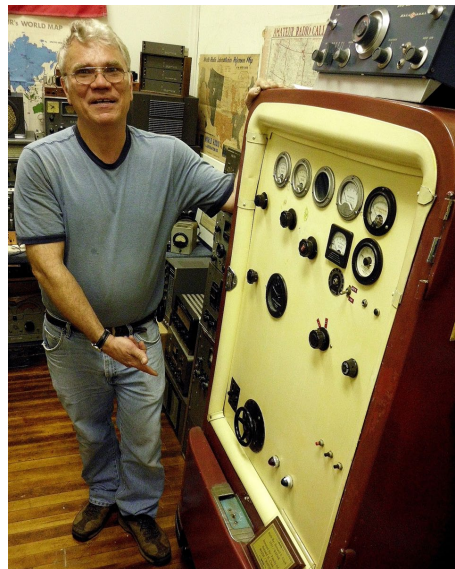
This ham radio transceiver was built by Bernard Clark W8PNR in 1953, using a refrigerator as a project enclosure.
