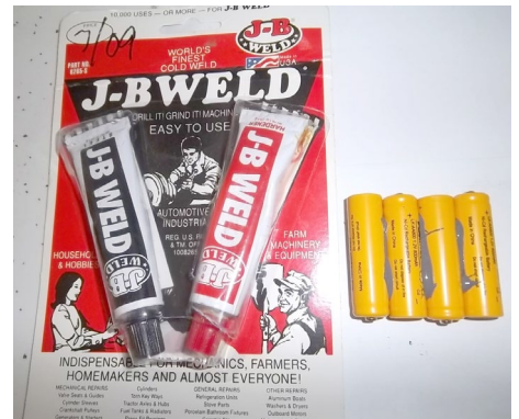
Photo 5. J-B Weld® used to glue the four NiCad cells together.
