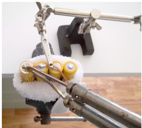
Photo 7. This little arrangement allows easy soldering. White tube sock cushions cells while in the vise. "Hands free" gizmo holds soldering wick in place.
