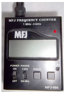
Photo 1. My trusty MFJ-886 Frequency Counter; a tool that is high on the totem pole of importance in my radio room.
