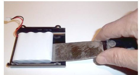
Photo 4. Trusty putty knife is used to gently separate pack from housing.
