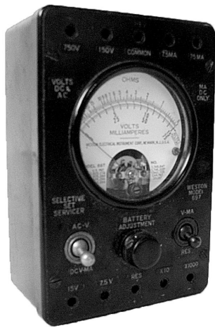
The palm-sized Weston 697 is a great help in diagnosing earlier radios, where voltage specs were given for 1000 ohms-per-volt instruments.
