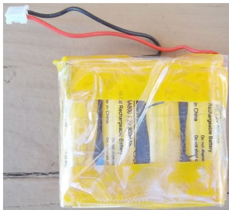
Photo 8. The final product: the completed NiCad pack replacement, ready to be installed in the unit. Since the batteries were yellow-colored I felt it only proper to use yellow electrical tape as an insulator.
