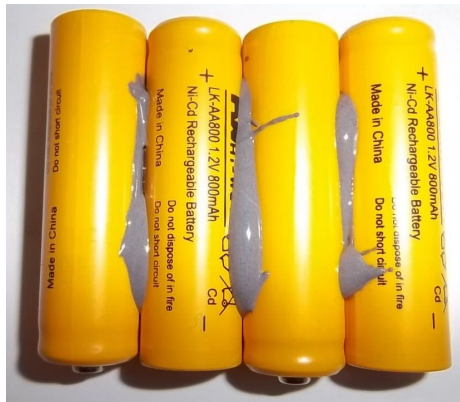
Photo 6. Four NiCad cells, glued together, and properly aligned in series and ready for soldering. Shiny gray material between the cells is the adhesive.
