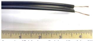
One version of TwinLead, a smaller balanced line of about 300 ohms impedance.
