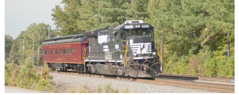
A minimal office car special, consisting of a Norfolk Southern engine and NS car 32, "Research." NS train 995-17 was en route from Roanoke, Va., to Raleigh, N.C., where, after a layover, the research car was added to an Operation Lifesaver special train. The old passenger car carries a variety of instrumentation for recording the performance of a variety of rolling stock.
