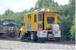
Front and rear views of Sperry Rail Services truck 983 at Huddleston, Va. The scanning equipment for detecting rail flaws is between the two highway tires. These trucks are set up so that they can operate in reverse while on the rails.
