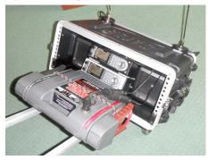
The metal enclosed speakers are Texas Rangers. They project very well and are warm sounding (not tinny) and can take the power of a small amplifier should you decide to add one. Power is derived from a rechargeable 12 volt/900 peak amp battery used in jump-starting cars.
