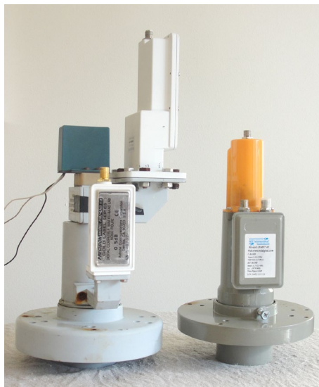
Traditional Chaparral international C/Ku-band feed horn (left) with C and Ku-band LNBFs, a total cost of over $300 vs WS DMX741 feed horn (right) with built-in C and Ku-band LNBFs, about $45. (Courtesy: Author)
