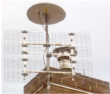
Photo 1. My antenna system, an omnidirectional mounted atop a 4-bay cage bidirectional. Both perform adequately for local reception and also serve up some TV DX when favorable conditions exist. Both have preamps to achieve decent reception.
