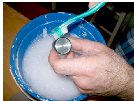
Cleaning the knobs made a real difference in the appearance of the set. A bucket of warm, soapy water and an old toothbrush made the job easy.
