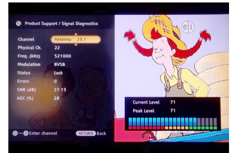
Photo 3. When purchasing a TV or converter box, check to see if it has a built-in signal strength meter, invaluable when aiming your antenna. The one below has the actual channel frequency, albeit in kilohertz, along with other useful information.
