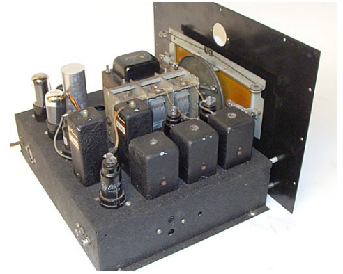
The "Broadcast 7" will be ready for re-installation in its cabinet once we take care of the sticking dial drive.
