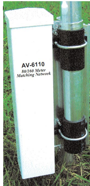
HyGain's AV-6110, a matching network that makes a 43 foot vertical actually WORK on 160 and 80 meters. (Photo courtesy MFJ Enterprises)
