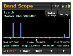
It's not in real time, but just so long as the span of spectrum isn't too wide, you have a good likelihood of seeing signals as they come and go. A press of a screen key allows you to hold and monitor the contents of any of those signals as they are discovered.
