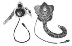
Fig. 4. At left, a carbon mic unit is installed in a noise reducing shield that was strapped over the user's nose and mouth. The same effect could be obtained (at right) by building the mic into an aviator's oxygen mask.
