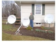
Author and his FTA satellite farm with three Ku band dishes. Left to right are: FortecStar 90cm motorized dish for satellites from 72W to 101W, middle is FortecStar 90 cm stationary dish mounted on a pallet pointed toward Hispasat (30W), yours truly, and finally a WS International 100cm motorized dish, for satellites from 15W to 61 W. I was able to optimize all these dishes much faster and easier with the Satlink WS-6906. (Photo by Edith Filippi)
