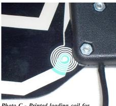
*Photo C - Printed loading coil for the VHF elements.*
