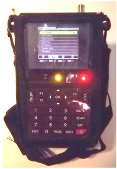
Satlink WS-6906, in the "On" position, with Power and 18V LEDs on. LCD display can be turned on and off using F1 key. Case and strap are useful when using outdoors to prevent scratching, and strap is used to hang unit around neck and prop against chest for easier viewing. Note that the carry case top flap can be folded over for easier viewing in bright light.
