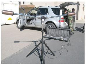
*Hi-Q Military portable HF NVIS antenna (Courtesy: www. hi-qmilitaryantennas.com)*
