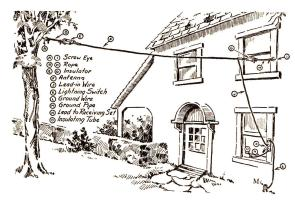
AN "INVERTED L" ANTENNA ADJUSTED BE A TREE AND THE WINDOW FRAME ADJUSTED BETWEEN
