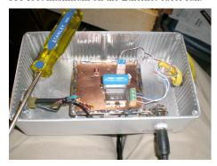
There is a standard 9 pin connector terminated on a cable for serial access. Connected to a serial port, you can download the integrated audio voltage level via a PC terminal program, such as *HyperTerm* in Windows XP. There is a nice freeware program out there that also works great called *WinPutty*.
