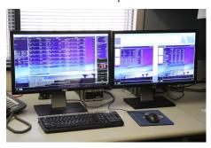
The dish operator monitors the various parameters displayed on the screens above. Note the DC power supply behind the Dell monitors. The monitors are run by highly regulated and filtered DC (direct current) power supplies in order to minimize RF (Radio Frequency) noise often associated with switching power supplies built into standard monitors.
