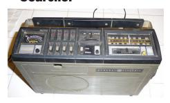
General Electric made just such a radio that is a nostalgic favorite of mine. Called The Searcher, this mid-1970's era portable radio offers coverage for the commercial AM and FM bands as well as four channels covering the VHF (Very High Frequency) Hi Band, noted on the radio itself as the Public Service Band (PSB). Each channel can tune independently between 150 MHz and 174 MHz via four tuning knobs located under a protective cover.
