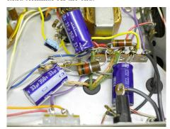
Parts placement for rebuild of power supply.
