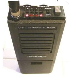
Crystal-based scanners could continuously check multiple frequencies, but the expense and mechanical effort necessary to add new frequencies put a limit on the dynamic flexibility of these units. Physical size and circuit board layout constraints also limited the number of crystals that could be accommodated, so there was an upper boundary on the total number of frequencies a scanner could support.
