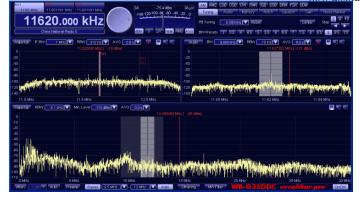
Three spectrum screens are shown in their default settings: the 0-30 MHz full-span spectrum analyzer (extendable to 50 MHz), and two, separate, smaller-span displays for more detailed analysis and recording.
