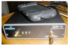
On the front panel, the yellow *CAP* light tells you're actively gathering data. The green *USB* light is lit when you are connected to the PC running software SDR-14 aware. The *CLP* (clipping) light comes on when you are overdriving the unit. You can set the preamp-gain to a more negative setting to reduce the gain. I used the -10 dB setting.
