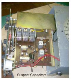
transformer; a pair of electrolytic capacitors (see Figure 2). Electrolytics are very prone to drying out and losing their effectiveness.
