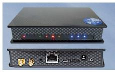
The audio output is via a 3.55mm stereo jack or it can be streamed over USB/Ethernet, and onto the Internet. The BaseStation software can also handle receiving ACARS digital signals using an audio port, but does require a separate ACARS decoder that is available as Freeware.
