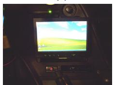
he used was to replace the control system with software that allowed the whole system to be tuned. To do this, he installed an in-dash PC that he bought from www.mp3car.com, one of several places from which you can buy PCs made for cars, as well as in-dash monitors, AM/FM receivers (to replace the functionality lost when you install a PC and/or a monitor in your dash), and more.
