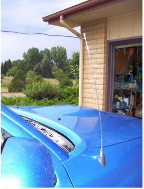
Photo 2. Replacement aluminum antenna mounted on truck with insulated wire running diagonally across the roof and into the bed of the pickup on the opposite side. The antenna bows slightly in order to make the wire as tight as possible.
