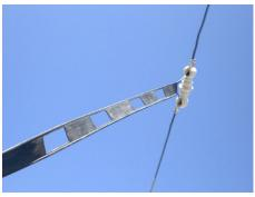
An old ceramic "dog-bone" insulator with smooth, well-rounded corners is probably the simplest way to connect 450-ohm window line to your antenna's feed point. The feed wires on WB0JNR's dipole go up and through the holes at each end of the center insulator to help relieve flexing stress, which can break soldered connections that aren't secured. (photo courtesy of Roger Wendell, WB0JNR, www.rogerwendell.com/mystation.html, of Golden Colorado)
