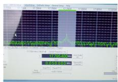
Photo 3. SpectraVue display showing an AM station being received at 17.7954 MHz. Audio from the SDR-IQ is sent back to the PC via the USB port, and played via the PC's sound card.
