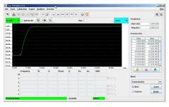
Figure 2 is a screen capture of the latest miniVNA software showing the spectral plot of the BCB filter from  $100\,$  kHz to  $5\,$  MHz. The filter exhibits classic high-pass characteristics, attenuating signals from 0- $1.3\,$  MHz by  $51\,$  dB. At  $1.8\,$  MHz signals are attenuated only  $0.4\,$  dB, and signals above  $2\,$  MHz or so are only attenuated by  $0.29\,$  dB. An exported plot of the same screen is shown in Figure  $3.\,$
