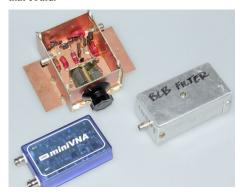
Figure 1 shows the miniVNA (about the size of a deck of playing cards) and two of the filters I evaluated while figuring out how to get the device up and running. At the top is the tunable 80-meter front-end filter from the W7ZOI/K5IRK Progressive Communications Receiver I've been "building" for 20+ years! It peaks desired signals between 3.5 and 4 MHz while attenuating unwanted signals outside that range.
