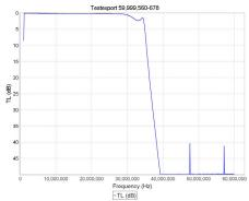
As shown in the miniVNA plot, the low-pass filter starts attenuating at 30 MHz, and by 40 MHz signals are chopped down by 50 dB (again, probably much more). The two spikes
