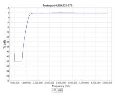
front-end filter. Notice that below 2.1 MHz and above 4.8 MHz, signals are attenuated by at least 51 dB (probably more). For a receiver that's designed to receive signals between 3.5 and 4 MHz, this is a good-performing filter. Thanks to the filter's variable capacitor, shown in Figure 1, the peak on the right-hand side of the passband is tunable between 3.3 and 4.3 MHz, and when a desired signal is properly "peaked," the filter's insertion loss is only about 3.5 dB. Nicel
