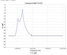
Figure 5 shows the response of my trusty Drake lowpass transmitting filter, designed to attenuate signals above 41 MHz by a whopping 80 dB. I know from experience that this filter works well. I forgot that it was inline one day and tried to work a station on 6 meters. My rig said it was putting out 5 W, but my external power meter read "no power." The filter, between the two, was doing its job!
