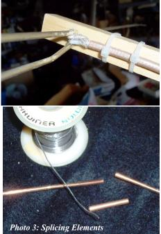
near, the voltage null, we keep RF off the coax shield. The coax center and shield connections need to be long enough to do the job and not much more.
