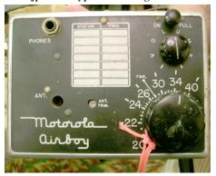
The Motorola Airboy: An example of an LF receiver used by aviators.
