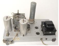
Fig. 3. The chassis top with the multisection electrolytic and i.f. transformers reinstalled.
