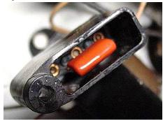
Fig. 2. With the potted capacitor removed, a modern unit can be installed in the Bakelite block. Gary Maker photo.
