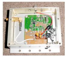
Photo E - Remounted PLL with Voltage Regulator
