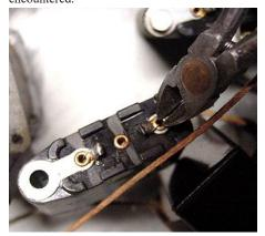
Fig. 1. First step in Gary Maker's Bakelite block rebuild procedure is to cut, at the terminal strip, the fine wires coming from potted components. Gary Maker photo.
