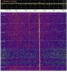
A screen capture using DL4YHF's software - Aircraft Doppler on 218 MHz.
