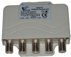
DiSEqC switch (\$13 plus shipping) connects up to four fixed-mount dishes to one run of coax into your house. Switching from satellite to satellite is done with the FTA receiver's remote control. (Courtesy: Sadoun Satellite)
