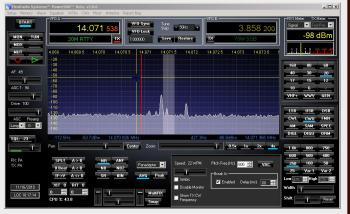
Modern band scope: Five signals on the digital subband on 20 meters as shown by PowerSDR on a day when propagation was down in the dumps. I wish I had made a screen capture during the Sweepstakes contest, as the band was packed with moderate to strong signals.
