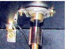
is done by attaching the three 1-1/4 inch long plastic standoffs to the bottom of each capacitor. A metal center point can be temporarily attached to the capacitor shaft with a shaft coupler. The point will accurately locate the height.
