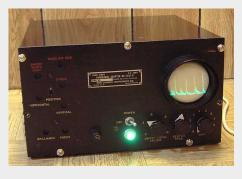
Classic band scope: This US Army Signal Corps BC-1031 panoramic adapter was used by Allied forces during World War II and later. An early spectrum analyzer, this BC-1031, built by New London Instrument Company, displays signals up to 100
