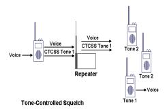
In our example, Users 1 and 2 would be assigned one CTCSS tone (tone #1) and Users 3 and 4 would be assigned a different CTCSS tone (tone #2). Their radios would be programmed to transmit the assigned CTCSS tone whenever they were talking and to listen for the assigned CTCSS when they were idle. So, when User 1 is talking, he or she is also transmitting tone #1.
