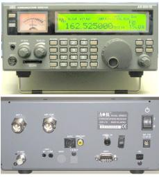
With continuous frequency coverage from 40 kHz-3150 MHz (3.15 GHz) (cellular blocked on the consumer model), this new receiver can search or scan (in voice- or mode-recognition options) as many as 2000 alphanumeric memory channels (in forty 50-channel banks).
