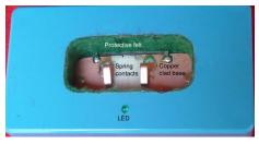
Figure 7. Charging base with interface contacts
