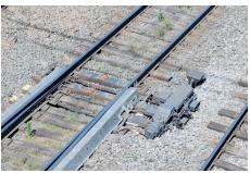
Power switch mechanism. This power switch is part of a cross-over, which in turn, is part of the Boylan Interlocking in Raleigh, N.C. The covered sheet metal channels outside the rails are part of the switch heater, which during precipitation in below-freezing weather, keeps the switch from freezing up or being blocked by ice or snow.
