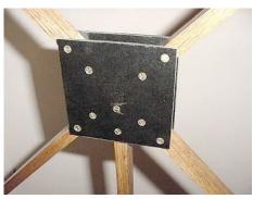
Detail of the center of the loop showing the square pieces screwed to the arms and mast.
