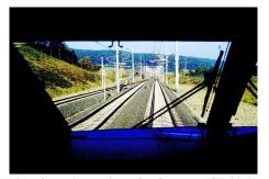
View from the engine of a German ICE highspeed train doing more than 150 miles per hour. This photo was made back in 1991! Note the continuous antenna running between the rails that is used to communicate data and instructions between the dispatching center and the train.
