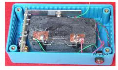
Figure 10. Bottom view with charger assembly in place
