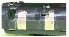
Figure 3. Contacts and diode in place
