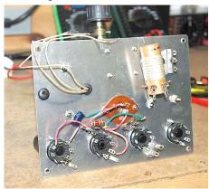
Construction itself took place over three or four days. Wiring and component placement was begun from the leftmost tube socket, which is the 35Z5 rectifier, and proceeded to the rightmost socket. Tools used were a needle nose pliers, variable temperature soldering iron, nippers, and something to hold and dispense solder.
