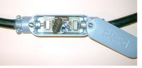
Figure 1. Photo shows Preamp circuit board mounted in conduit body (Photo by Kevin Carey)
