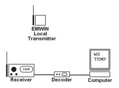
NWS broadcasts EMWIN over two satellites, called GOES East and GOES West. GOES East can be found in the Clarke Belt at 75 degrees West and GOES West at 135 degrees West. Together they provide coverage for the North American continent. EMWIN data are transmitted up to both of these Geostationary Operational Environmental Satellites from a NOAA facility on Wallops Island in Virginia. The 9600-baud data stream comes down from both satellites at 1690.725 MHz.
