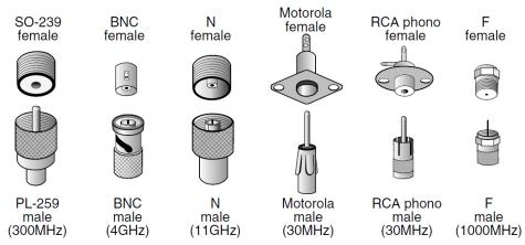
The most common antenna connectors and their maximum recommended frequencies.
