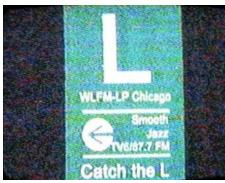
This 3kW station in Chicago simulcasts audio with an FM radio station. WLFM-LP, Channel 6, was received via E-skip at 735 miles. (Courtesy: Author)
