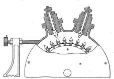
Fig. 3. Synchronous gaps required special generator power supply, tended to be used in commercial installations.
