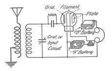
Fig. 4. Grid leak circuit offered detection and amplification in a single tube.
