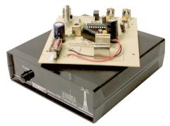
Ramsey Electronics' FM10C Part 15 transmitter (Courtesy: Ramsey Electronics)
