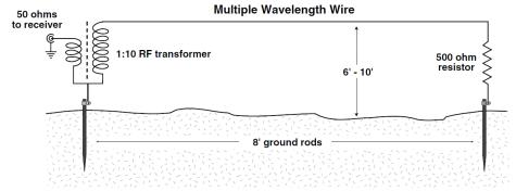
The Beverage is an example of a high performance, low frequency, grounded receiving antenna.
