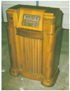
A 1941 Philco model 41-285 the "McArthur Set", as some call it. The original finish bleached, breached, and rubbed with oil by a well-meaning person. Knobs gone and escutcheon warped beyond help. Good starting material, though.
