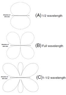
A halfwave dipole (A) as seen from above has a classical figure-eight pattern at right angles to the curve. The same antenna at twice the frequency, now a full wavelength, has a cloverleaf pattern.
