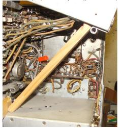
BC-344 power supply has to be propped out of the way to get at lower i.f. adjustments.
