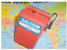
A Galcom solar-powered receiver fix-tuned to WRMI's frequency of 9.955 MHz.
