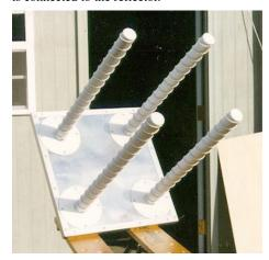
To the casual observer, a helical antenna appears as one or more "springs" or helixes mounted against a flat reflecting screen. The length of the helical element is one wavelength or greater. The reflector is a circular or square metal mesh or sheet whose cross dimension (diameter or edge) measures at least 3/4 wavelength. The helical element has a radius of 1/8
