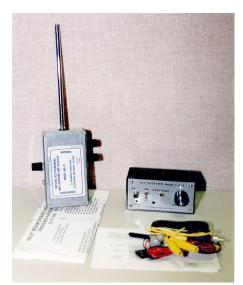
Figure 1. The WR-3 (left) and L-500L are two Commercially Made Natural Radio Receivers. (Photo by K. Carey)
