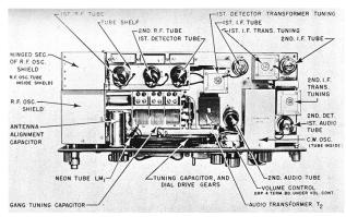
Fig. 4. Looking Down at the Top of the Radio
