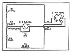
Fig. 1. Schematic of the S20-R "S"-Meter
