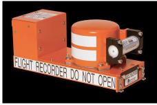
An example of a combination CVR/FDR unit. The cylindrical structure on the end is the Underwater Locator Beacon (ULB) which can send pings once per second for a month down to depths of 14,000 feet when activated by submersion in water. Photo courtesy L3 Communications
