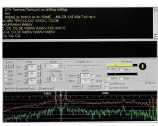
Typical RTTY screen shows the distinctive twin peaks of a RTTY signal, in this case, RK6CK, Temyruk, Russia. (Courtesy: Author)
