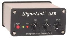
Tigertronics' SignaLink USB (\$100) is a compact digital interface that comes with a CD of software for the most popular digital modes including PSK31, SSTV, CW, RTTY, AMTOR, and Packet. (Courtesy: Tigertronics)
