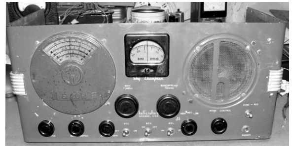
After a workover with rubbing compound and with its knobs detergent-cleaned, the front panel has a much fresher appearance.
