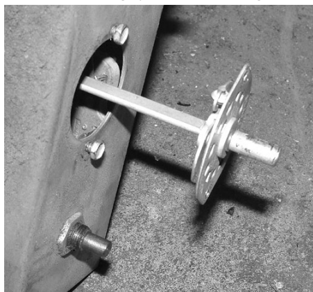
Bandswitch shafts are easily withdrawn from switch wafers, making it convenient to replace shaft damaged by drilling with shaft from parts set.
