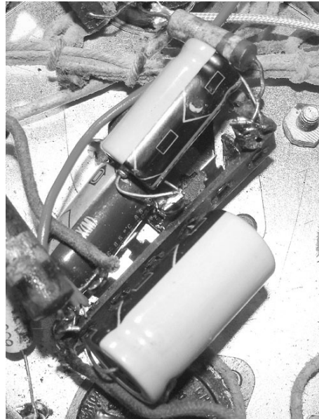
Thanks to their compact size, the new electrolytic caps could be shoehorned into the space under the original multi-section can.
