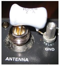
If you make the measurement at the end of a length of coax, you must subtract the coax distributed capacitance from the displayed value. The coax capacitance is revealed on the display before connecting the capacitor.
