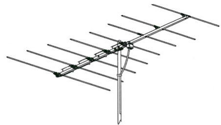
Winegard's HD6055P 10 element FM antenna (Courtesy: Winegard)
