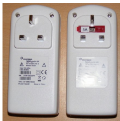
This picture is of the exact model PLC units that caused the problems in the UK. Someone was advertising them on the internet as from their BT Vision kit. In all complaint cases, the British Ofcom has simply required that they be taken off the air.
