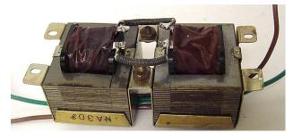
Fig. 1. Isolation transformer made from two low-voltage transformers with secondaries connected (see text).
