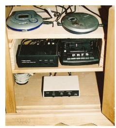
The author's personal broadcasting facility consisting of a low-power, limited-range AM transmitter plus MP3, CD, and audio cassette players and a Radio Shack audio selector. From here, replays of Golden Age radio material can be broadcast to an assortment of vintage radios scattered around his house.
