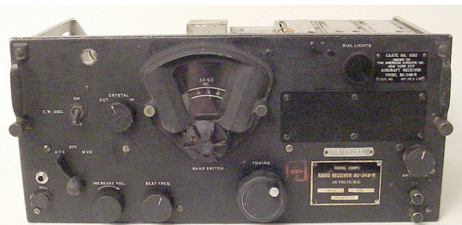
With knobs installed, front panel is now virtually complete. Hole at upper left, made by previous owner for a fuse, may eventually accommodate a fuse holder or a send/receive switch.
