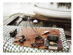
John also comments that "These sets (AOR AR8200 and AR8600) thrive on discone antennas, which, being inefficient below 25 MHz (with vertical frequency extender), don't overload them. At my base set-up I use the 8200 from 530 kHz up. Can occasionally receive such toughies as R. Sondergrense 3320 and Oz N Territories on 2310, 2325, 2485 kHz.
