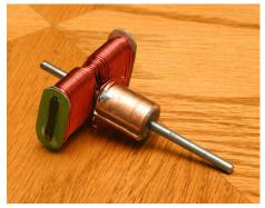
Figure 7. Completed armature with commutator connected by soldering.
