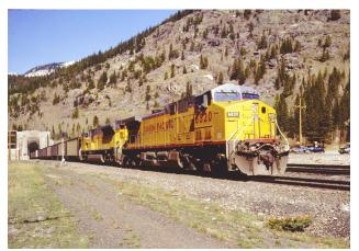
The same eastbound Union Pacific train described above in a more wide-angle view. The loaded coal train from the Craig Branch in western Colorado has additional sets of locomotives in mid-train and at the end, all of which will help in dynamic braking on the way down to Denver.
