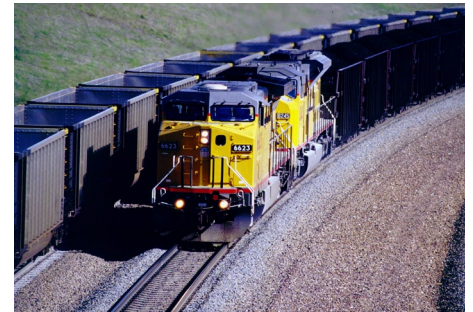
Outbound (southbound) loaded Union Pacific unit coal train passing an inbound empty train at Logan Hill on the south end of the Orin Line in southeastern Wyoming. The plastic dome on the lead locomotive protects an antenna array, including the one needed for remote control of other locomotives further back in the train.
