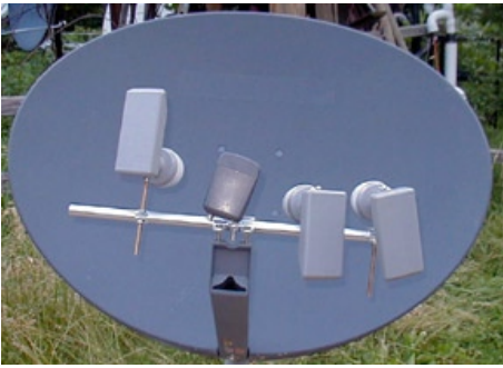
Multi-feeds for your Ku-band dish allows reception of several satellites. Switching is done with a DiSEqC switch. (Courtesy: Global Communications)
