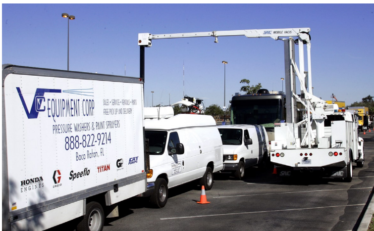
All the vehicles headed into the secure area of Dolphin Stadium are swept by the mobile VACIS or Vehicle and Cargo Inspection System. (Courtesy DHS Customs & Border Protection)
