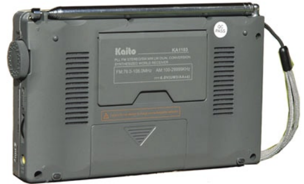
View of KA1103 back panel shows retractable desk stand, built-in, swiveling 36" telescoping whip antenna and battery compartment. Also seen from this view is the main tuning control, clarifying thumb wheel, line out jack, narrow/wide audio selector and front panel light switch (helps save on batteries when not plugged into the wall). (Courtesy: Kaito USA)
