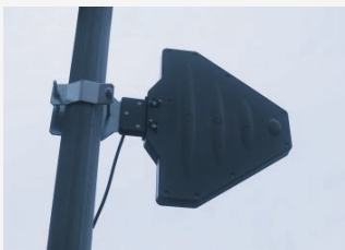
WR-AX-37E Directional UHF log-periodic antenna
