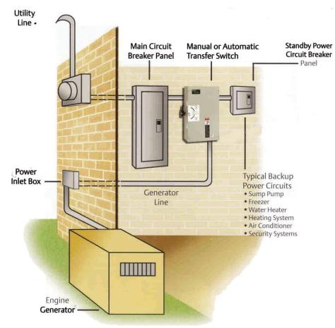
rity system, and other equipment. Upon utility failure, the user will need to start the generator. After the generator has warmed up, the homeowner will then position the manual transfer switch to the generator source. The manual transfer switch quickly breaks connection on the utility then quickly makes contact with the generator.
