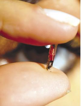
passive. All are capable of transmitting whatever they're programmed to send. Some can be reprogrammed. Active tags have built-in power supplies which power their tiny transmitters while passive tags use the power transmitted from the tag reader to transmit back the programmed data on their miniature antennas.
